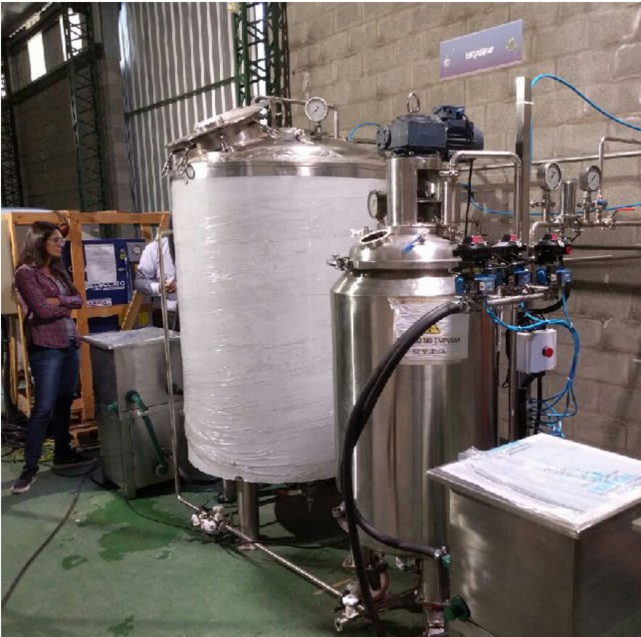
Illustration 3: The 200 and 1000 lt fermenters, in revision before the final tests.
