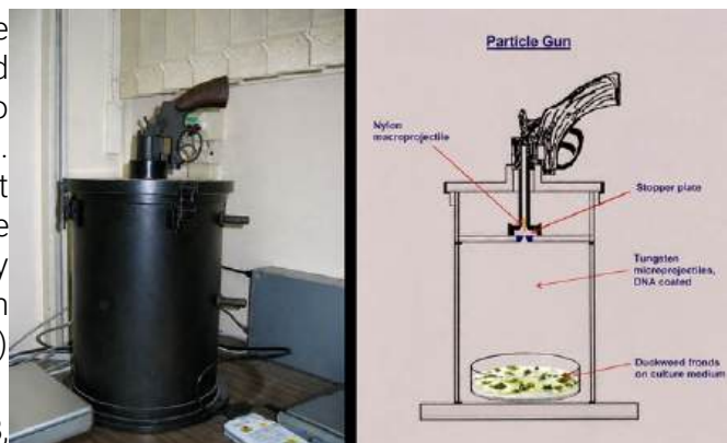
Figure 1: Early particle gun for duckweed transformation with Duckweed Plant illustration (Edelman group, 1990).
