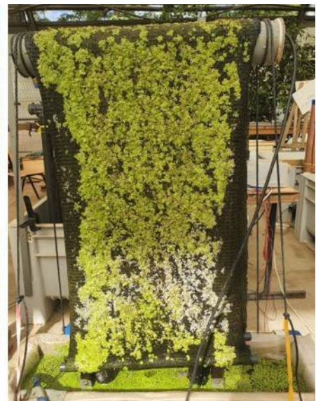
Figure 1: Prototype of an innovative vertical Lemnaceae cultivation system. Left, schematic overview of the system. Right, system in operation at Ein Shemer.
