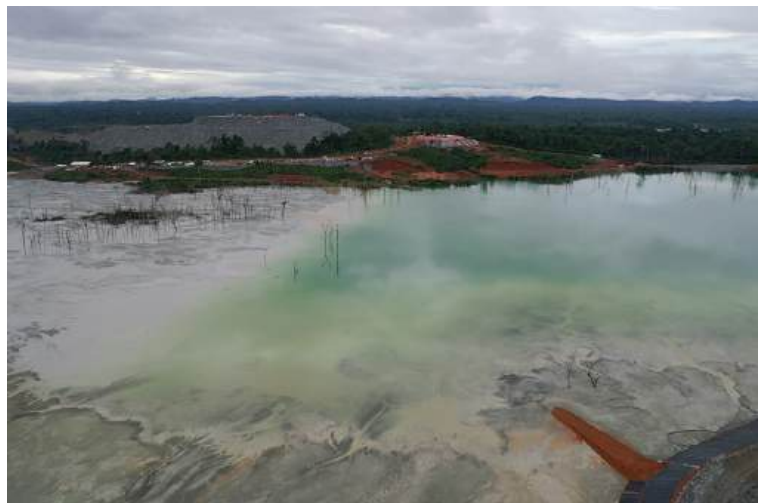
Figure 3: Drone imagery of the Tailings Storage Facility (TSF) of New Liberty Gold Mine
